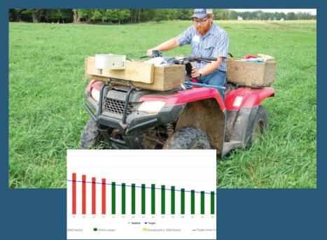
This device takes 50 readings per second to measure the forage height.
